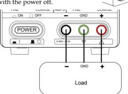
2. Set the current and voltage knobs to the left most position (0A, 0V).
