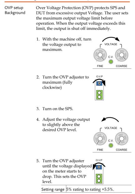
Note Over voltage protection is always on and cannot be disabled. The OVP voltage however, can be set to the rating voltage +5.5%.
